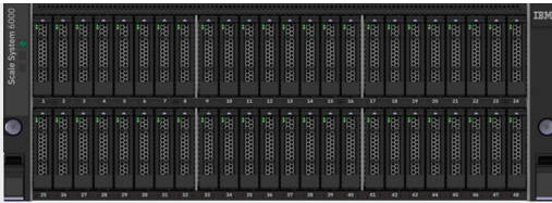
Figure 4 – The IBM Storage Scale System 6000 can store 1.44PB of uncompressed data in a single 4U rack configuration and can scale to yottabytes.
